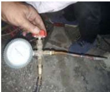
Fig.3: Leakage test rig for brazing fitted with pressure gauge
